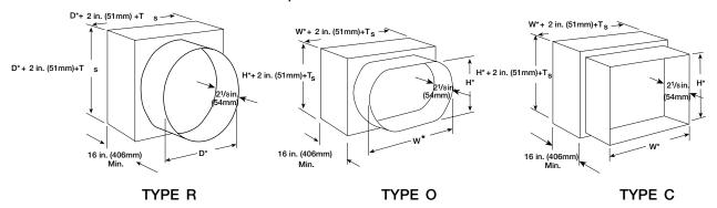
\* These dimensions are furnished approximately 1/4 in. (6mm) undersize, except round and oval dimensions which are approximately 1/8 in. (3mm) undersize.
